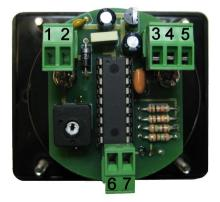
Whenever power is applied to the unit, the meter needle will swing to 10 with the WheelSlip Indicator on, and back to zero with the OverSpeed Indicator on. This is so you can observe that everything's working.
